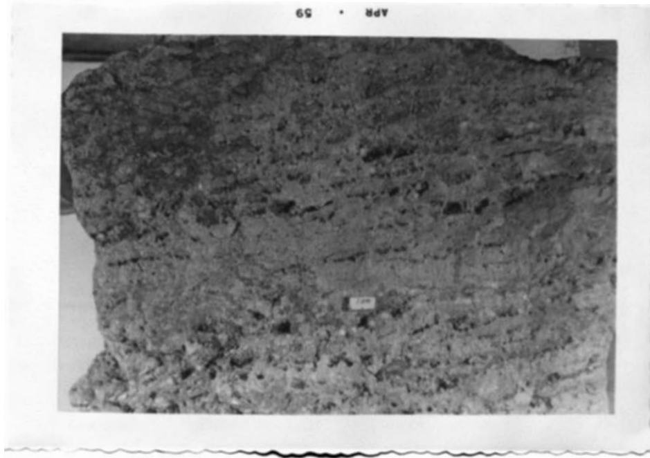
Figure 38. Hand specimen with galena in dolomite taken from the dumps at the old Annapolis Lead Mine. Note the bedded nature of the vugs and the galena. Galena occurs in many of the vugs and as bedded disseminations.
